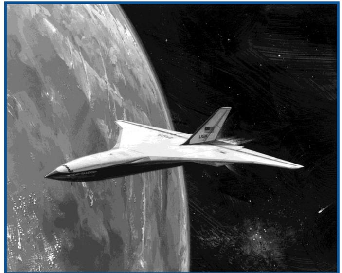
**Above:** The use of reusable launch systems is revisited in the 1970's by Rockwell International with their Star-raker concept. The HTOHL, single-stage-to-orbit design made use of 10 Mach 6-capable turbo-ramjet engines for atmospheric flight and 3 liquid-propellant rocket engines for orbital flight. Large for its time, the Star-raker had a 360 foot wingspan and payload capacity near 200,000 pounds.
